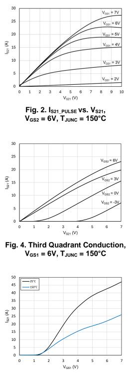
Fig. 6.  $I_{S21_PULSE}$  vs.  $V_{GS1}$ ,  $V_{GS2} = 6V$ ,  $V_{S21} = 10V$
