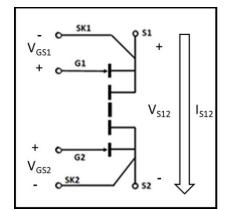
Fig. 1.  $V_{GS1}$ ,  $V_{GS2}$ ,  $V_{S12}$ ,  $I_{S12}$  Definition (Note 1 - 3)
