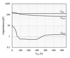
Fig. 12.  $C_{ISS}$ ,  $C_{OSS}$ ,  $C_{RSS}$  vs.  $V_{SS}$ ,  $V_{GS} = 0V$
