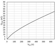
Fig. 14.  $Q_{OSS}$  vs.  $V_{SS}$ ,  $V_{GS} = 0V$
