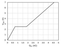
Fig. 9.  $V_{GS1}$  vs.  $Q_{G1}$ ,  $V_{GS2} = 6V$
