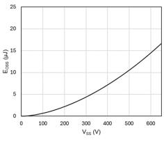
Fig. 16.  $E_{OSS}$  vs.  $V_{SS}$ ,  $V_{GS} = 0V$
