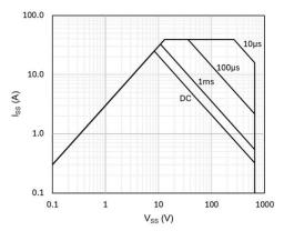
Fig. 19. Safe Operating Area, T<sub>JUNC</sub> = 25°C
