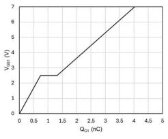
Fig. 10.  $V_{GS1}$  vs.  $Q_{G1}$ ,  $V_{GS2} = 0V$
