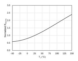
Fig. 8. Normalized R<sub>SS(ON)</sub> vs. T<sub>JUNC</sub>
