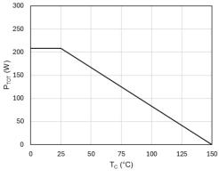
Fig. 17. PDISSIPATION VS. TCASE
