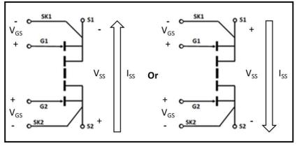
Fig. 3. V<sub>GS</sub>, V<sub>SS</sub>, I<sub>SS</sub> Definition (Note 4 - 6)
